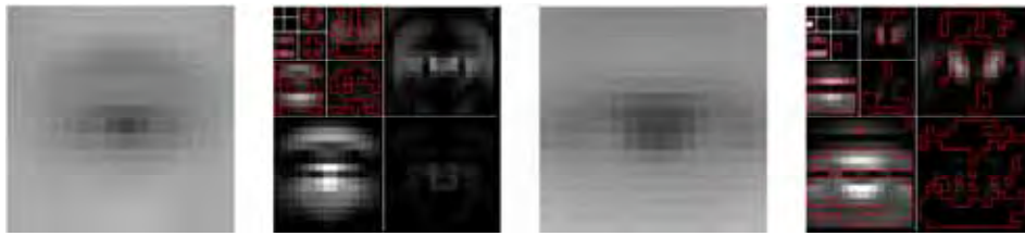
Figure 6. From left to right: the mean eye pattern, its wavelet decomposition and the selected features (red contour) of the two eye patterns. High intensities correspond to strong edges, low intensities indicate uniform regions
