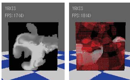
Fig. 4. Simulation of fire and smoke on the billboard. The fluid animation is simulated on a 64x64 grid billboard.
