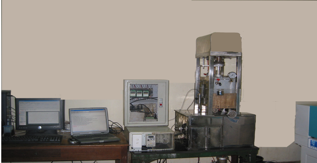
Photo 1 Three-axial dynamic cycling loading test equipment
