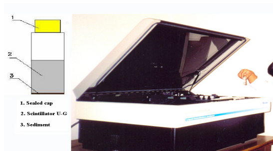
Fig. 3. Measurement the total beta radioactivity by LSA Tri-carb 2770TR/SL.
