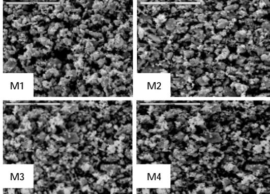
Fig. 4. SEM Images of isotropic bulk samples M1-M4 sintered at  $1260^\circ\text{C}/2\text{h}$  (bright line is  $10 \mu\text{m}$ ).
