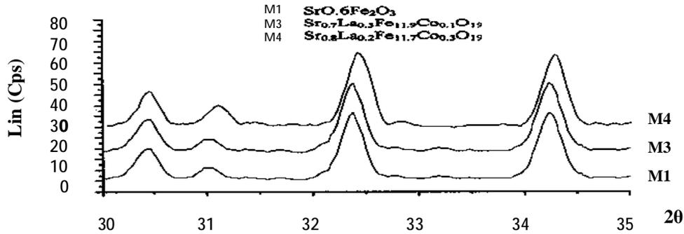
Fig. 3. X-ray diffraction patterns of the samples M1, M3 and M4 sintered at 1260°C/2h.
