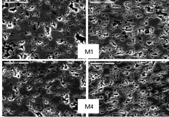
Fig. 5. SEM Images of anisotropic bulk samples M1, M4 perpendicular (left) and parallel (right) to the preferred magnetizing direction (bright line is  $10 \mu\text{m}$ ).
