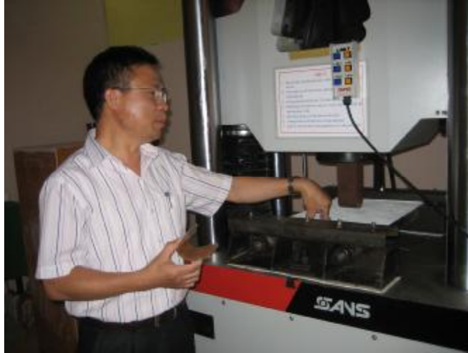
Fig. 1. Bending test for 3-phase composite plate.
