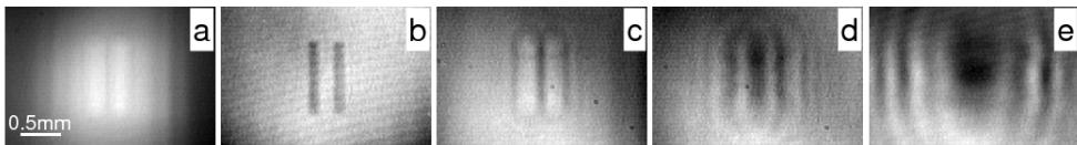
Fig. 11. Experimentally observed 2D interference patterns in the scheme of Fig. 10. [(a)-(e)]: the double slit is placed at the positions of  $z_{01} = 31.0, 28.5, 24.2, 20.0$ , and  $10.6$  cm, respectively, where (b) is the image of the double slit (Zhang et al., 2009b).
