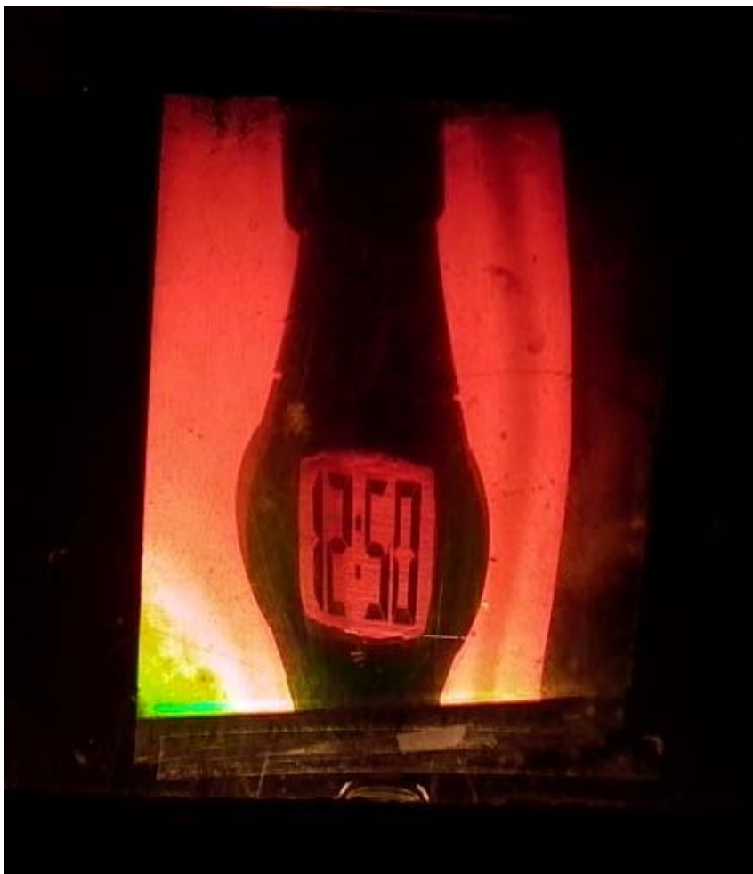
Fig. 11. A LCD transmission watch as seen in the linear source projection
