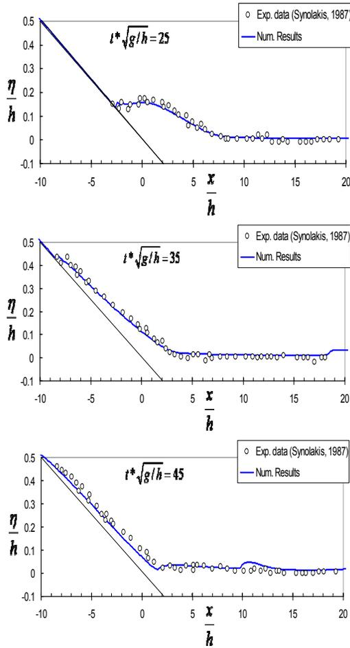
Fig. 4. Comparison with experimental data: runup phase.
