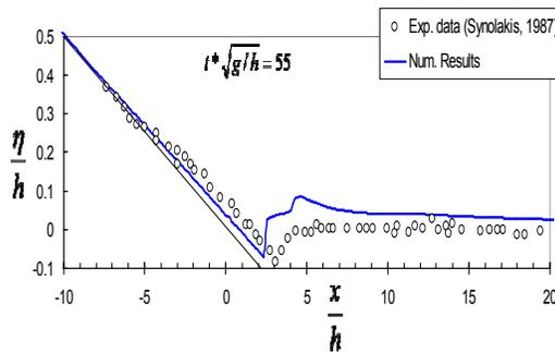
Fig. 5. Comparison with experimental data: rundown phase.
