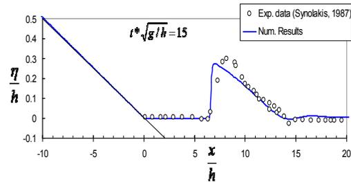
Fig. 3. Comparison with experimental data: near breaking location.
