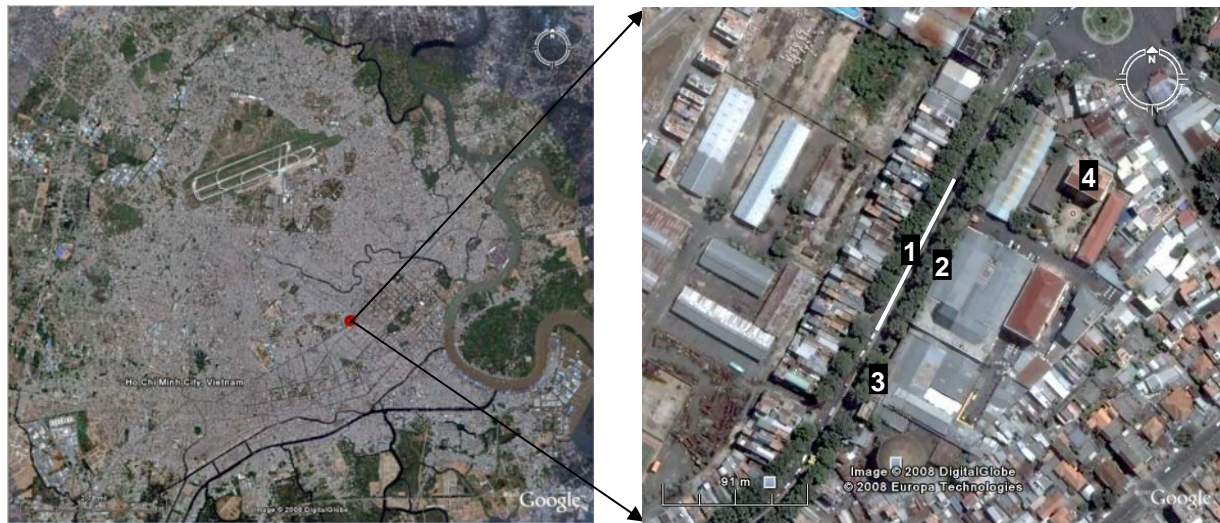
Fig. 1. The survey site (left: in HCMC map; right: in 3/2 Street, 1: Emission liberation device; 2: Mobile station; 3: Traffic video recording; 4: Weather station).
