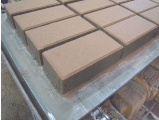
Figure 3 Production of satisfactory eco-paving blocks
