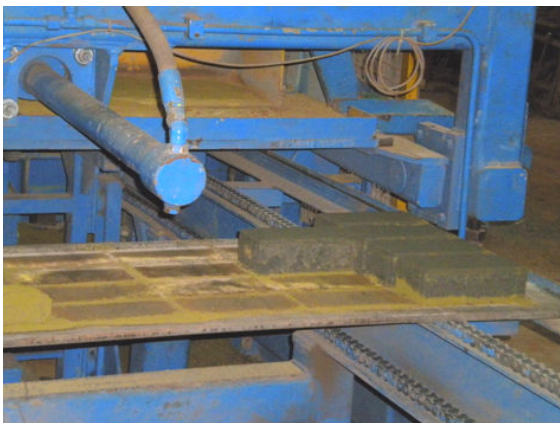
Figure 4 Production of eco-paving blocks of poor yield rate and quality
