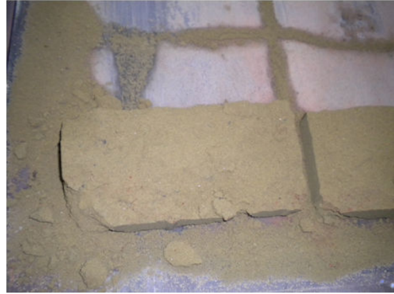
(a) Very poor mixing within whole matrix
