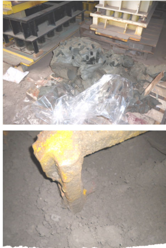
Figure 1 Wet marine mud and mixing (lumps of marine clay are seen, poor mixing)
