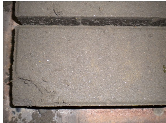
(b) Non-uniform mixing with poor edge
