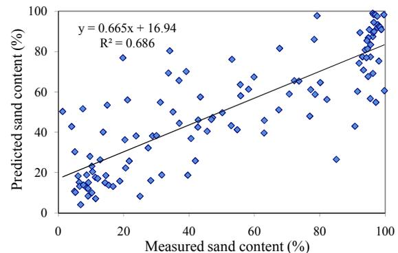
Figure 6 Scatter plot of predicted and measured sand contents in sediments.
