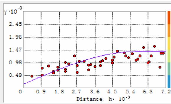
Figure 5 Empirical semivariogram (circles) and spherical model (continuous line).
