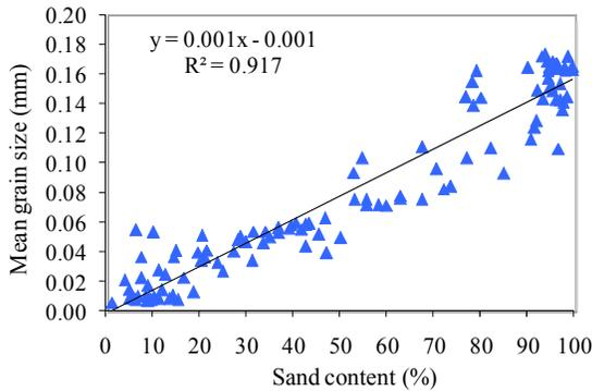
Figure 4 Scatter plot of mean grain size and sand content of sediments.
