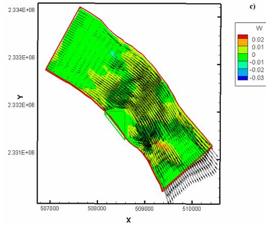
Figure 3 Velocity field at the surface layer
