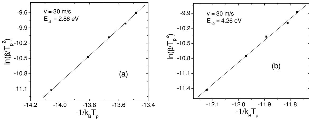
Fig. 3. Kissinger plot of sample  $v = 30$  m/s, the first peak (a) and the second peak (b).
