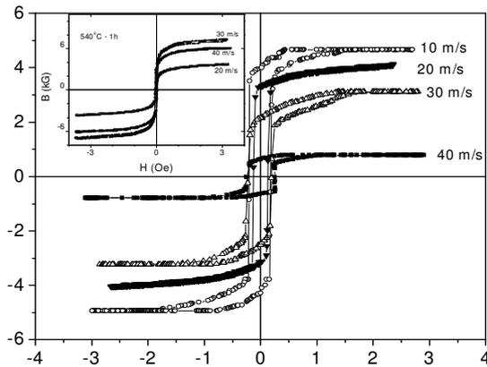
Fig. 6. Hysteresis loops of as-spun samples and samples annealed at 540°C for 1h (insert in Fig).
