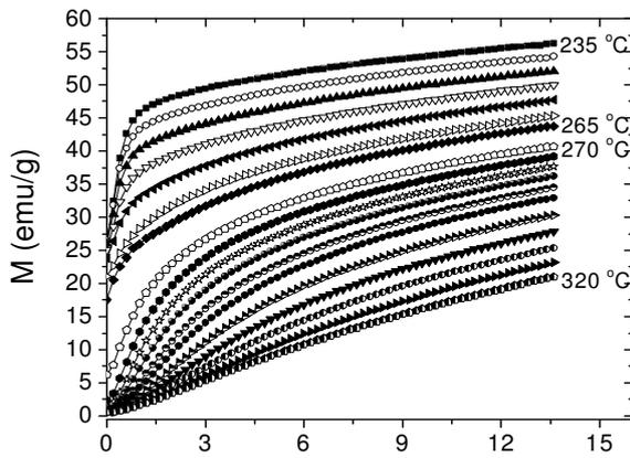
Fig. 7. Isothermal magnetization curves of sample with  $v$  of 30 m/s measured at different temperatures around  $T_c$ .
