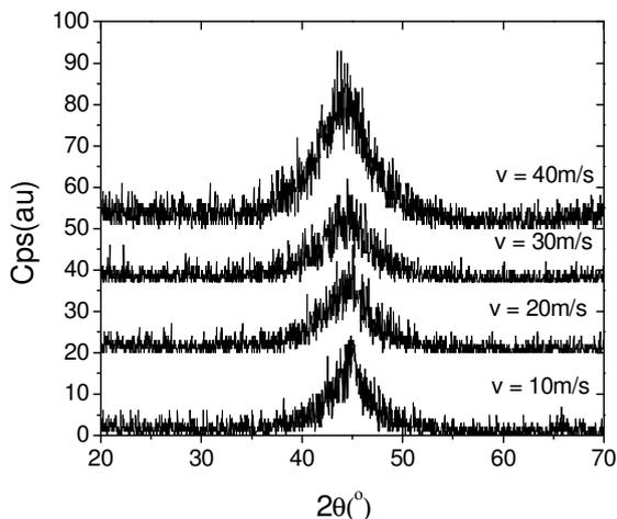
Fig. 1. X-ray diffraction patterns of as-spun ribbons  $\text{Fe}_{73.5}\text{Si}_{13.5}\text{B}_9\text{Nb}_3\text{Au}_1$ .
