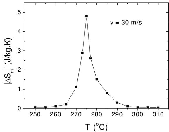
Fig. 8. Magnetic entropy change versus temperature in  $Fe_{73.5}Si_{13.5}B_9Nb_3Au_1$  with  $v$  of 30 m/s in the field change  $\Delta H = 1.35$  T.
