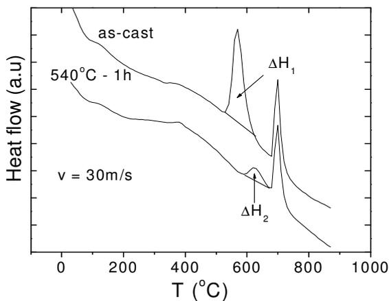
Fig. 4. DSC curves of as-spun and annealed ribbon with  $v$  of 30 m/s.
