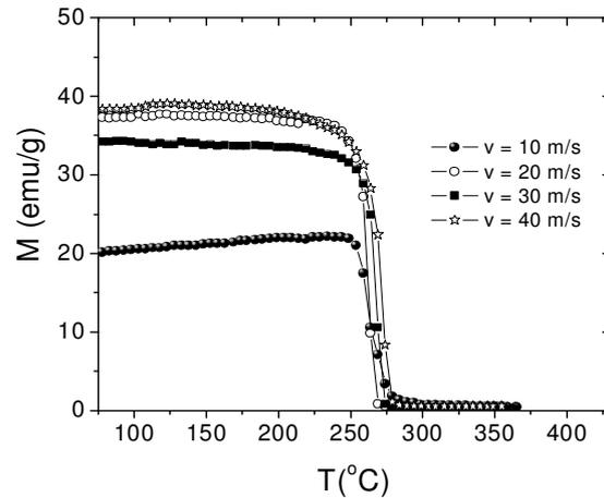
Fig. 5. Thermomagnetic curves of the studied samples measured in the field of 20 Oe .
