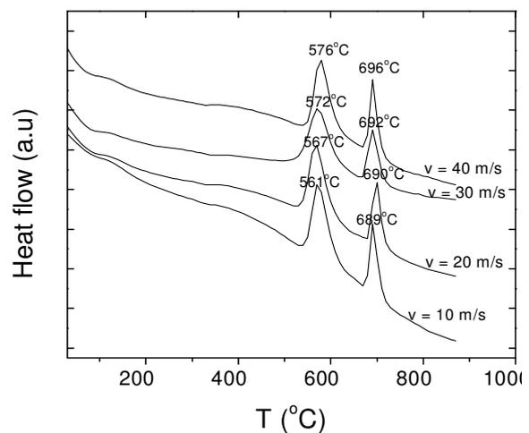
Fig. 2. DSC curves of the studied as-spun ribbons with heating rate of  $20^{\circ}\text{C}/\text{min}$ .
